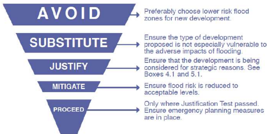
Figure 2 Sequential approach principles in flood risk management
