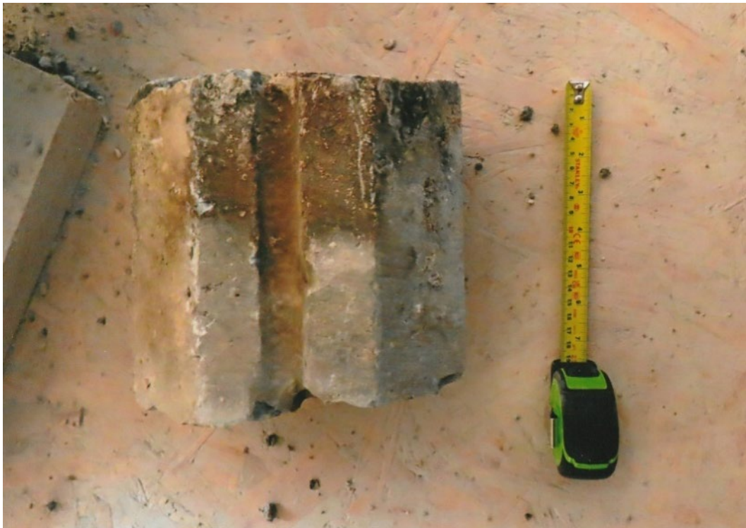
Fig. 38 Side view of the window mullion fragment. Photograph: J. Higgins.
