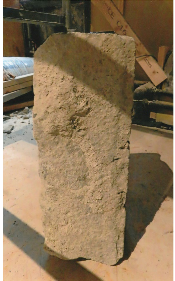
Fig. 21 A&B Two sides of an ashlar block with a thin coat of 1950's – 1960's cementitious shuttering from the ground floor window of the south transept extension. The ashlar block is probably of the 14th to 15th centuries. Photographs: J. Higgins.
