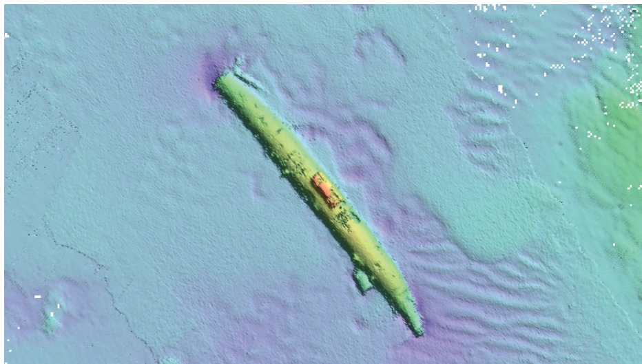
Multibeam image of the wreck of the German UC-42 submarine, lying on the sea-bed off the coast of Co. Cork. This is one of many such images produced by the INFOMAR project, which is mapping the sea-bed around the coast of Ireland and it highlights the benefits of collaborations between agencies (Image courtesy of INFOMAR/Geological Survey Ireland/Marine Institute).
